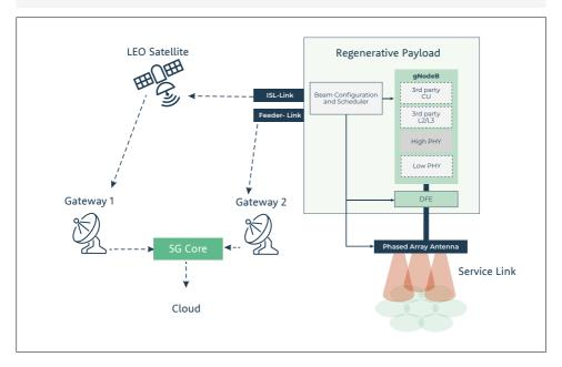
The regenerative architecture requires that a large amount of real time signal processing is carried out on the satellite, which effectively becomes a base station in space. The onboard environment of a satellite brings with it requirements that are very different from those in which terrestrial base stations operate. In particular, Size, Weight, and Power (SWAP) are all tightly constrained.
